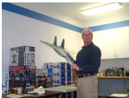
Don Wood's showing his scratch built F-14 foam aircraft. He built it using Depron foam painted with polyurethane. Operational swing wings add a scale touch. According to Don it flies well. If it flies as well as it looks it must fly great.
